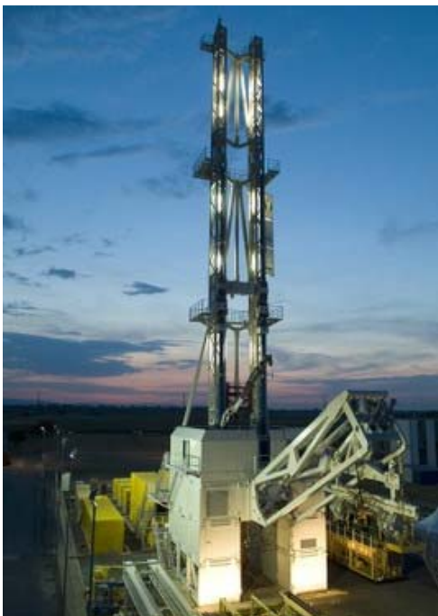
Figure 3: The Innova Rig, an innovative drill rig for science and exploration serves as a test bed for the TRIDEC Drilling use case.
